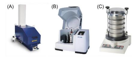
Milling system. (A) Crashing mill. (B) Planetary ball mill. (C) Analytical sieve.
