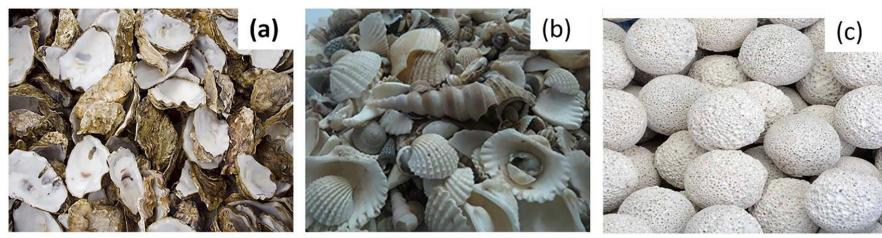
Typical biofilter media from waste shells for wastewater treatment: (a) oyster shells; (b) mixed waste shells biomaterials; and (c) shaped waste shell powder
