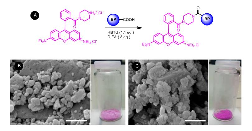
A) Reaction of functionalization of the oyster shell particle (BP) with the rhodamine B (Rho-B) piperazine molecule. B) SEM image of bleached oyster powder (shown in the vial) after chemical functionalization with Rho-B. C) SEM image of the pristine oyster powder (shown in the vial) after chemical functionalization with Rho-B. Scale bar is 1 μm.
