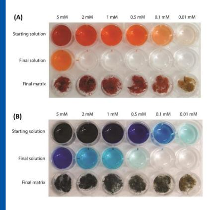
Camera photographs illustrating the dye removal experiments using (A) de-metaled byssus on EosY solutions, and (B) native byssus on MB solutions.
