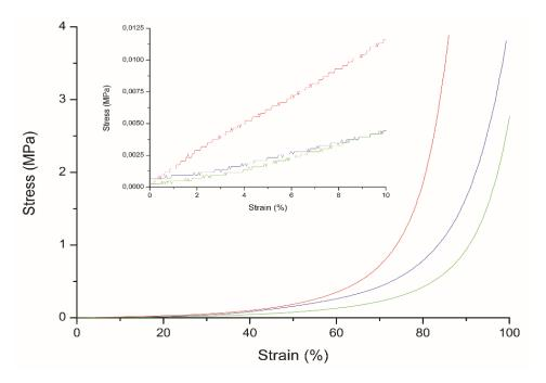
Uniaxial compression tests on the three different matrices: in red the metal-treated matrix, in green the native matrix and in blue the EDTA-treated matrix. Inset: A zoom in the 0-10% strain region.
