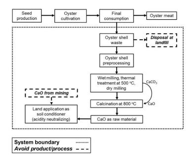
System boundaries of the processing and reuse of oyster shells
