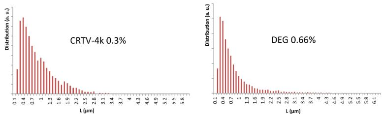
Particle size distribution of bCC after planetary ball milling grinding in the presence of different grinding aids, polyacrylic super-fluidificant CREATIVE 4K © (CRTV) and di-ethylene glycol (DEG).
