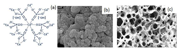
Structure of hydroxyapatite (HA) biomaterial: (a) molecular structure  $[Ca_{10} (PO_4)_6 (OH)_2]$ ; (b) scanning electron microscope image of HA powder; and (c) porous microstructure of HA.
